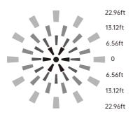
Mounting Height <12m/39.37ft Ceiling Mounted Detection Distance Radius 3-7m/9.84-22.96ft
